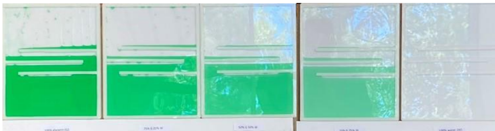
Figure 1 - Five enclosures at rest, from L to R, colored glycerin, 75%-25%, 50%-50%, 25%-75% glycerin-water mixtures, and water.
