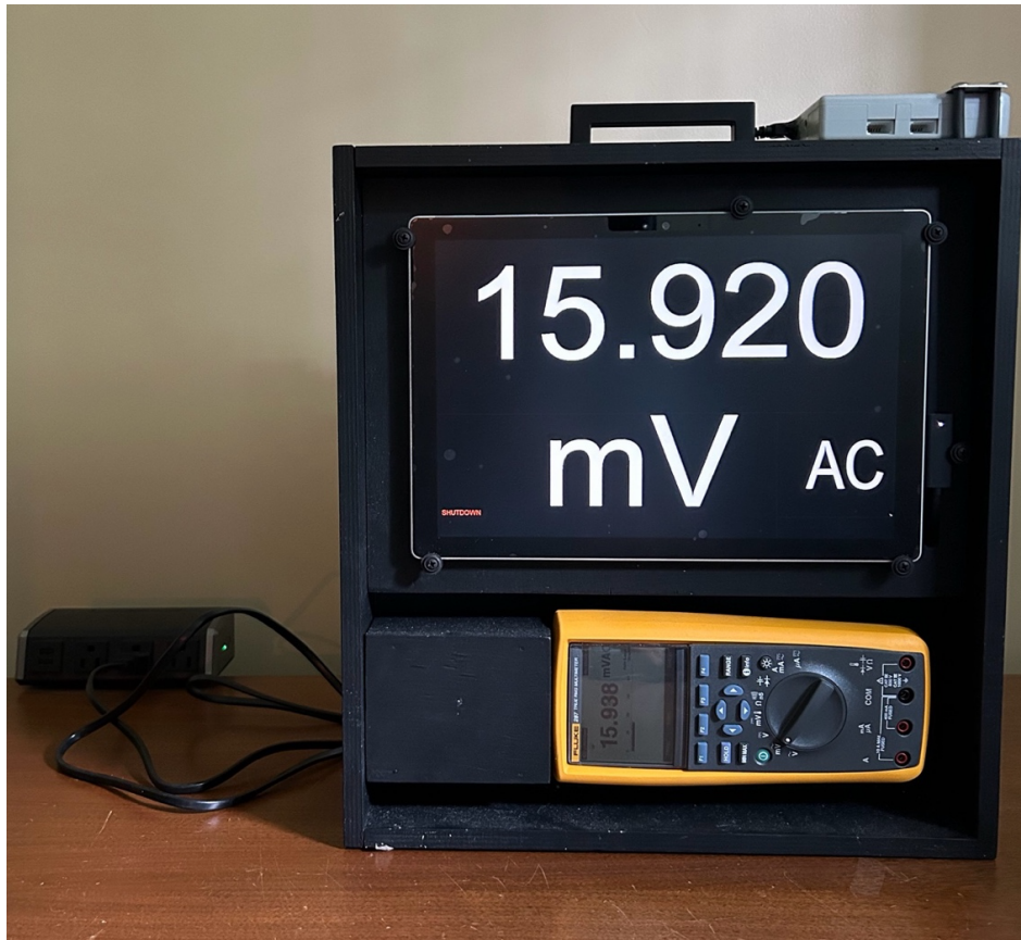
Figure 1: Front of device. Ignore the Labquest mini mounted at top. A U-shaped piece of wood hides the cable coming out of the multimeter. The computer is an old Surface Pro 4. There is an approximately 60 millisecond delay in communications between the Fluke and the computer, which is normally not noticeable unless a still shot is taken as above, where the Fluke has already moved on to the next measurement while the previous voltage is still shown on the computer.
