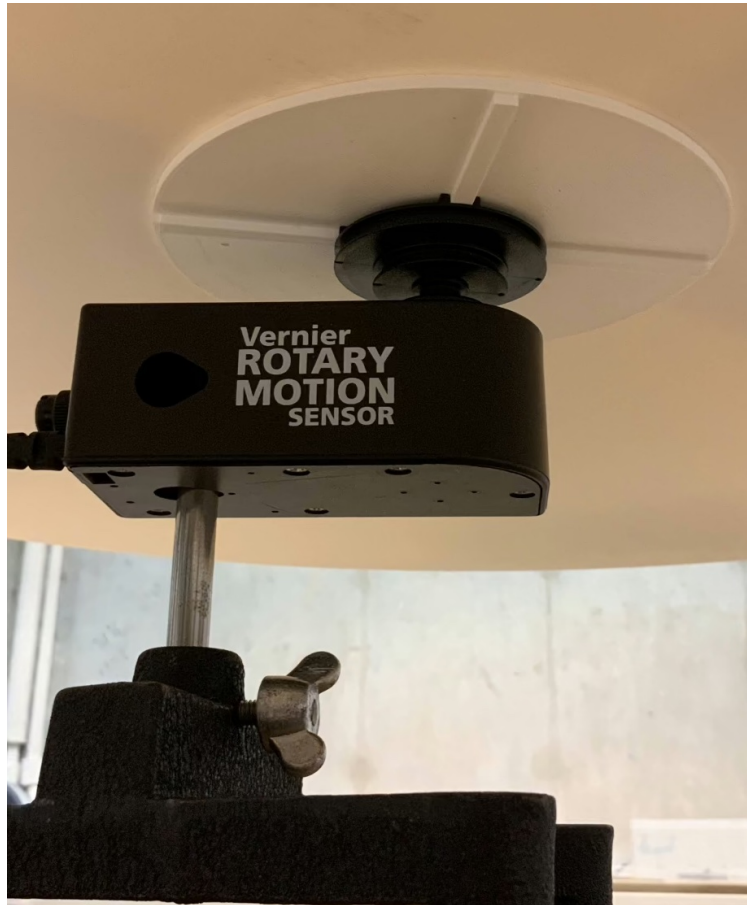
Figure 2: The underside of the turntable. A 3D printed part provides some additional support to the foam core turntable. An additional smaller disk of foam core could also be used.
