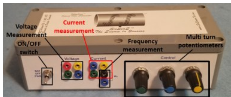
Figure 2. The set of plugs shown in the above figure are used to measure voltage across each LED, the current they are subjected to and the light intensity (frequency measurement) at the fiber tip .
