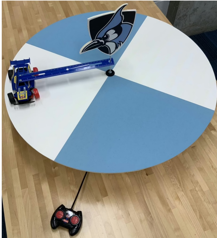
Figure 1: The assembled angular momentum apparatus.
