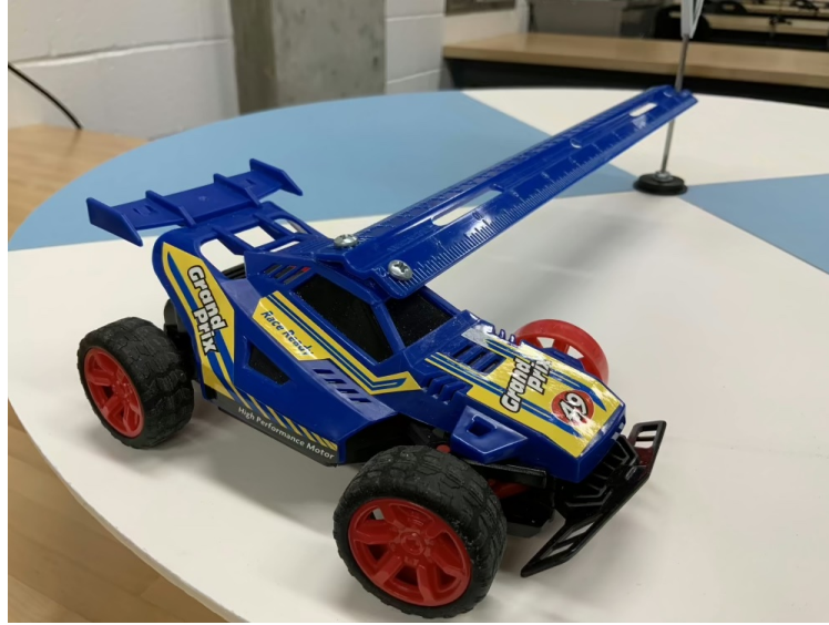
Figure 3: The car is constrained to rotate in a circle by the ruler. The inside tires are removed so that the car drives more uniformly in the tight circular trajectory – the toy car is not equipped with a rear wheel differential.
