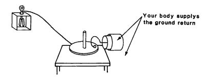
4. Once it is established that the system will hold charge, carefully lift the insulated plate a small distance. The leaves of the electroscope will separate more. When the insulated plate is lowered, the leaves will return to their original position. Carefully move the insulated plate sideways without changing the separation between it and the lower plate. As long as the plate does not get too near the edge, the leaves of the electroscope will remain unchanged.
