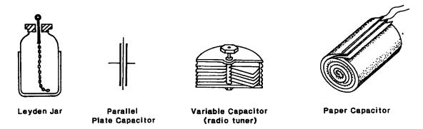
One plate of a capacitor is connected to the source of electrons, such as the negative terminal of a battery. The second plate is connected to the positive terminal of a battery. Electrons will accumulate on one plate. This creates an electric field which then repels the electrons on the other plate causing them to flow to the positive terminal of the battery. The process continues until the potential difference across the capacitor is equal to the potential difference of the battery.
