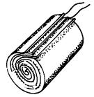
Changing the area or thickness of the dielectric, or changing the dielectric material itself will affect the capacitance of the device. In general:
