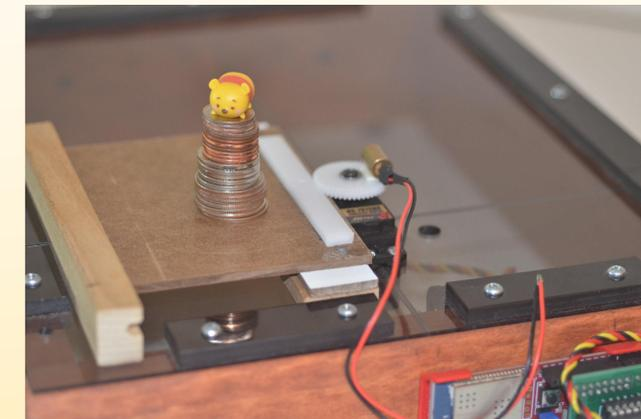
Our "Function Plane" is simply a servo motor mounted with the chipKIT control board on a wood and plastic box.
