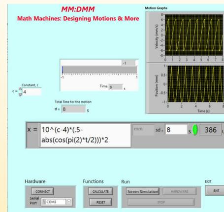
Distributed as a free LabVIEW executable, the interface allows learners to program physical motions directly with Excel-like algebraic formulas. Functions can specify either  $x = f(t)$  or  $v = f(t)$ . The software can also replay (in original or modified form) data sets such as the waveforms recorded by digital seismometers..
