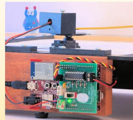
We use a Digilent chipKIT WF32 with a micro-SD card, a shield and a sketch that let users store and rapidly play very large sets of position (or RGB color) data. The sketch can control a hobby servo motor, a stepper motor, a low-power laser or an RGB LED.
