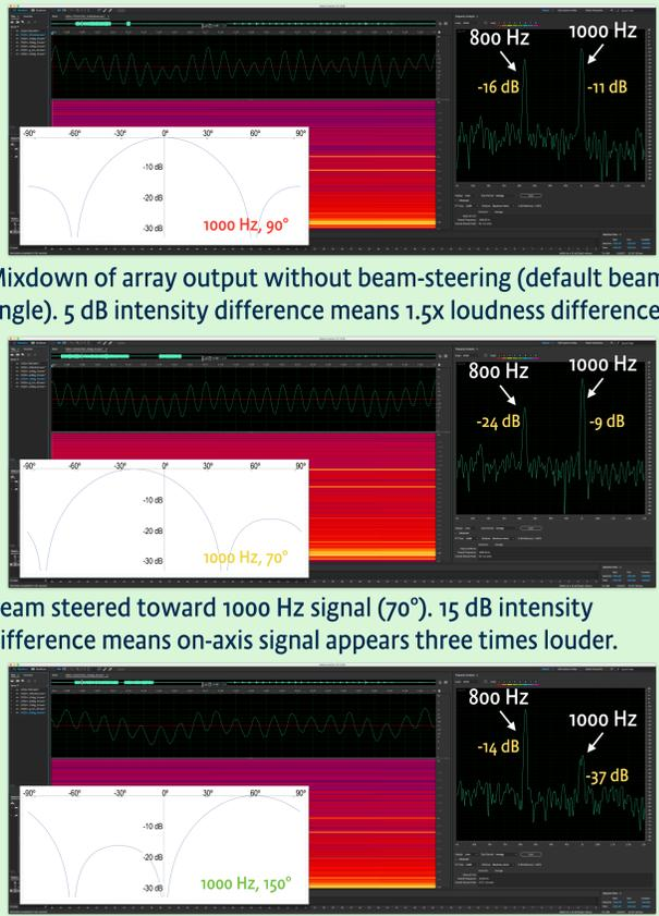
Mixdown of array output without beam-steering (default beam angle). 5 dB intensity difference means 1.5x loudness difference.
