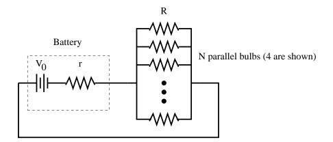
The battery is connected to N identical lightbulbs in parallel. The bulbs each have a fixed resistance R, independent of the current through them.
