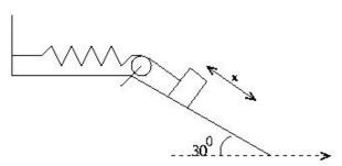
Assume that all surfaces are frictionless and that the pulley is frictionless as well.
