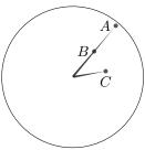
The three points shown on the clock hands have accelerations of magnitude  $a_A$ ,  $a_B$ , and  $a_C$ . The point B is at the midpoint of the long hand. Which of the following is true?
