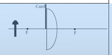
Image Formation Demonstration 3: What will happen to the image if you block the top half of the object with a card? Answer in words and show what happens on the diagram on the right by making any changes needed in the rays you drew above for Demonstration 1.
