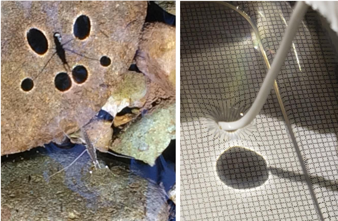
Fig. 2: Left: Image of a water strider on a water surface, demonstrating the shadows caused by the fluidic lenses produced by the water strider's legs. Right: A Polytetrafluoroethylene (PTFE) coated wire used to simulate a water-walking insect's leg on a water surface, lowered on to the surface using the height apparatus. Note the shadow at the bottom of the container and the distortion of the grid lines by the fluidic lens.
