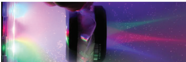
Figure 12: The red, green, and blue light from the LED array passes through the concave air lens. The light gets focused and an image of the color LEDs is formed to the right of the concave air lens. There are some distortions since the LEDs are outside the tank.
