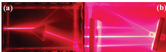
Figure 15: (a) Red Laser beam getting refracted by a prism in the scatter tank. Note the part of the beam that is reflected at the prism interface. (b) Combination of a 10 cm focal length convex lens and a 10 cm focal length concave mirror placed in the scatter tank.
