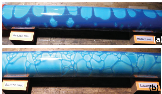
Figure 2. (a) Interaction of soap and air bubbles in annulus enclosure, (b) Plateau borders seen in annulus enclosure. Blue food color was added to the white soap.
