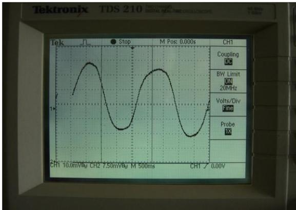
Hold the thermistor near your open mouth while you inhale and exhale to produce an oscilloscope display similar to that in the photo above.
