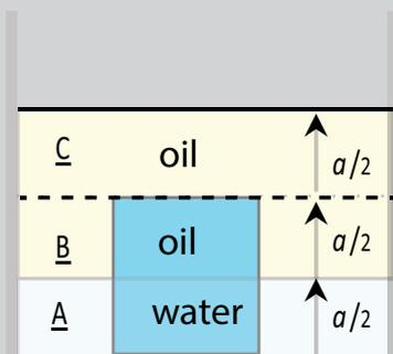
Since the density of each object/region is uniform, its center of mass (COM) is located at its geometric center, as shown in the table below.
