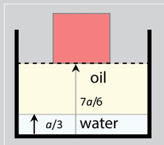
The positions of the centers of mass of cube, water, and oil in this final configuration can then be calculated, as shown in the table. (We will assume that the densities given are *weight* densities.)
