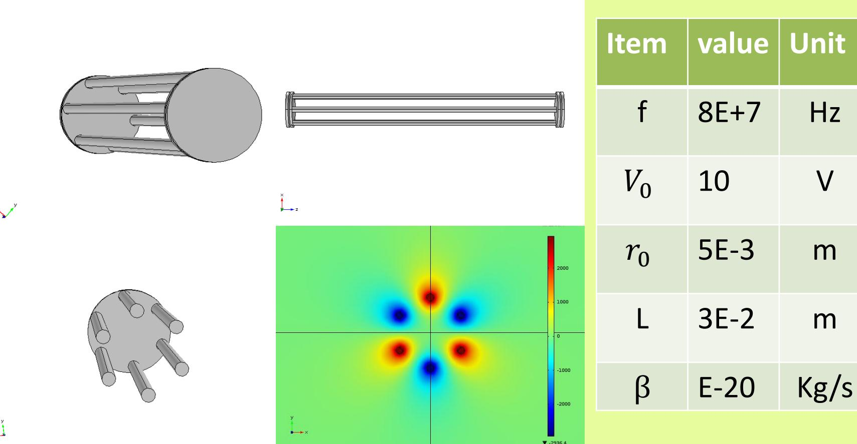
$$\text{Electric Potential inside the trap: } V = \frac{V_0 \sin(wt) \cos(n\varphi) r^n}{r_0^n} = \frac{V_0 \sin(wt)}{r_0^n} X(r, \varphi)$$
