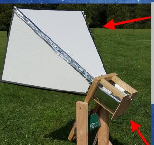
Stand - constructed from 2" x 2" and 2" x 4" wood
