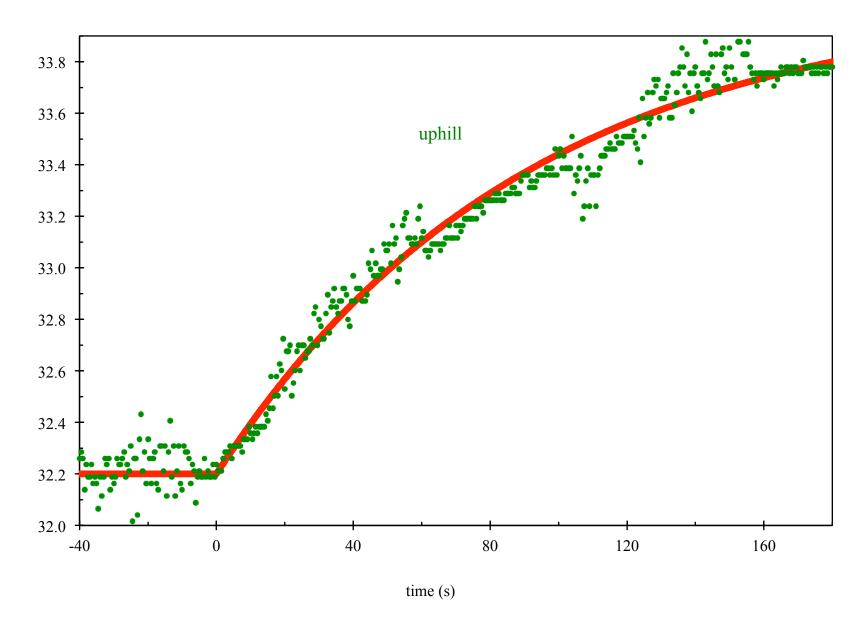
Based on Newton's law of cooling, fit the saturating exponentials shown as the red curves.
