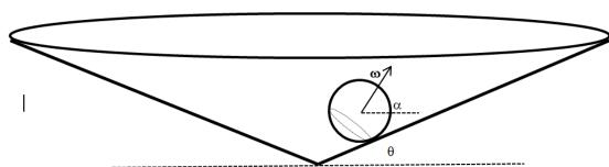
$$R_0 \dot{\phi}_{orbital}^2 = gh_0' / \left( 1 + \frac{I}{ma^2} \frac{\cos(\alpha)}{\cos(\theta)\cos(\alpha - \theta)} \right)$$
