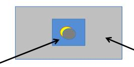
Using a shadow of a target on the frame, the telescope is adjusted to follow the position of the sun. The region around the sun is monitored continuously.
