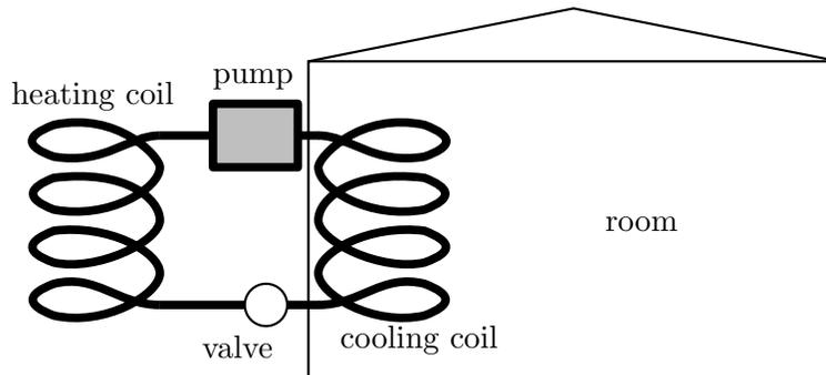
Assume that the outside air temperature is  $T_H$  and the inside air temperature is  $T_L$ . The air-conditioner unit consumes electric power  $P$ . Assume that the air is sufficiently dry so that no condensation of water occurs in the cooling coils of the air conditioner. Water boils at 373 K and freezes at 273 K at normal atmospheric pressure.
