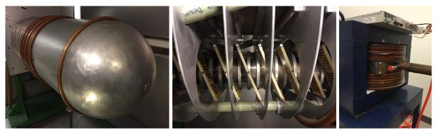
Accelerator dome (assume it is a sphere); accelerating column; bending electromagnet
