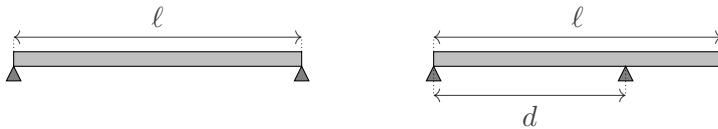
Suppose a rod is supported at both ends, so that it forms a bridge, as shown at left above. Assume the supports are simple, so that they only provide an upward force, and no bending moment. In equilibrium, a bending moment will appear throughout the rod. The magnitude of the maximum bending moment the rod can exert at any point without breaking is  $M_0$ , and the length of the rod is  $\ell$ . The bridge is loaded uniformly, with a mass per length of  $\lambda$  (including its own mass).
