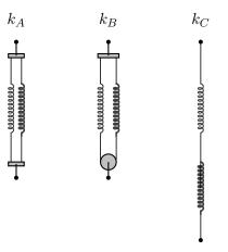
In the second case, the springs are connected to opposite ends of a string, which runs under a massless frictionless pulley. In each case, the two springs act like a single spring with an effective spring constant  $k_A$ ,  $k_B$ , or  $k_C$ . Which of the following is correct?
