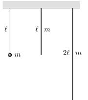
What is the correct ranking of the moments of inertia  $I_1$ ,  $I_2$ , and  $I_3$  about the pivot points?
