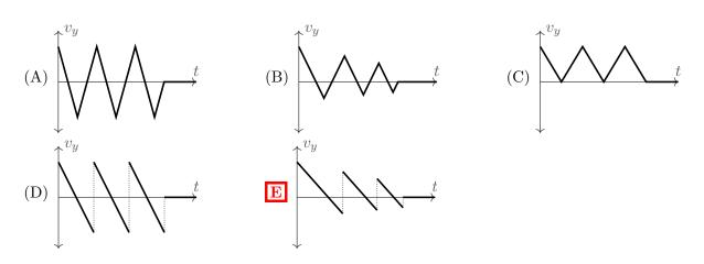
Since gravity provides a uniform acceleration downward, the graph of  $v_y$  should be decreasing with constant slope everywhere except at the collisions, ruling out all but choices (D) and (E). The collisions provide the discontinuities. To decide between the two, we note that the typical vertical velocities shown in the figure get smaller as the ball nears the top, so the correct choice is (E).
