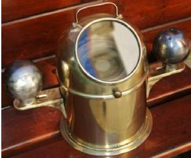
A binnacle, protecting the ship's compass in the center, with two soft iron spheres to help correct for errors in the compass heading. The use of the spheres was suggested by Lord Kelvin.
